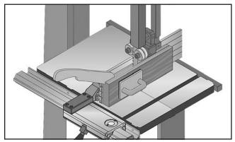
Figure 54. Example of a resawing operation.
